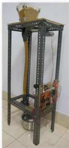
Fig. 6: Laboratory setup for detecting seed flow in a delivery tube.
