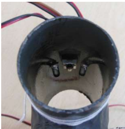
Fig. 3: IR LED and TSOP receiver fitted inside a 'Y' pipe.
