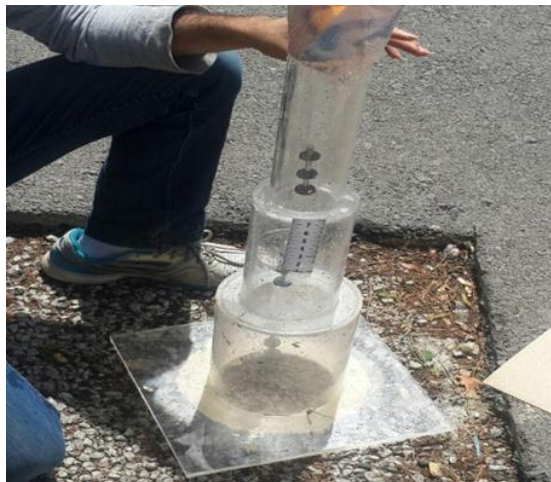
Fig. 2: A Gilson device built for measuring permeability.
