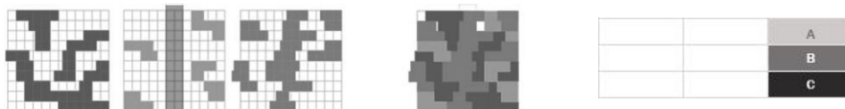
Fig. 4: Basic arrangement of living units, from left to right, level A, level B, level C, superimposed ABC(elevations) and a Site schema highlighting area being discussed (Top view of structure).
