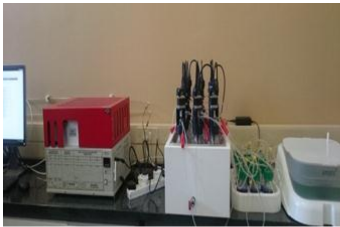
Fig 3: Biogas Production set-up from left to right, Gas Chromatograph, Digesters, CO 2 , Collection bath
