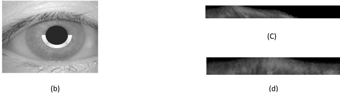
Fig. 4 : a) Architecture of normalization using BCA. b) Quarter iris region. c) Rectangle template that generated using BCA before scaling process. d) Rectangular Iris generated after scaling process with height 45 pixel and width 240 pixel of the quarter iris region.
