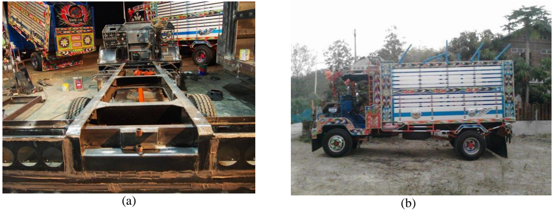
Fig. 1: Agriculture truck superstructure; (a) Chassis frame, (b) Pick-up structure
