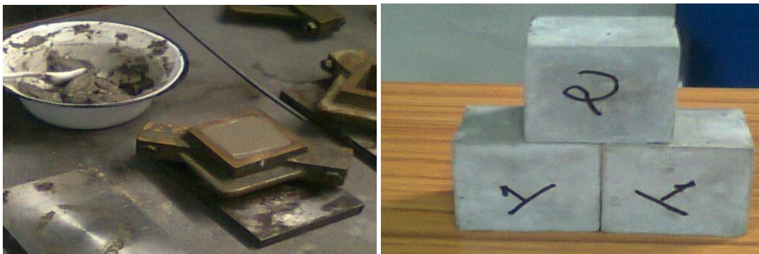
Fig. 2 & 3 Casting of Geopolymer cubes
