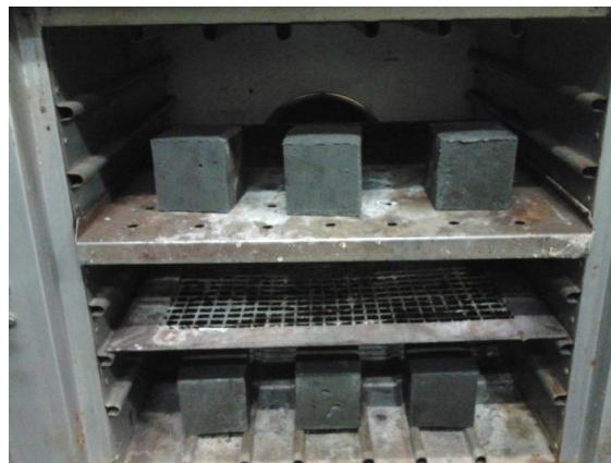
Fig. 4 Heat Curing of Geopolymer Cubes
