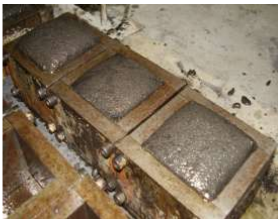
Fig. 3: Expanded aerated concrete before trimming
