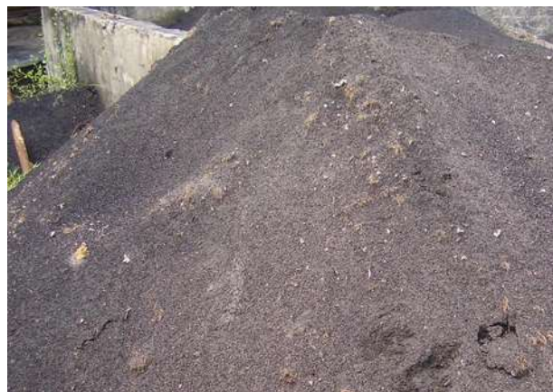
Fig. 2: Palm oil fuel ash dumped as waste
