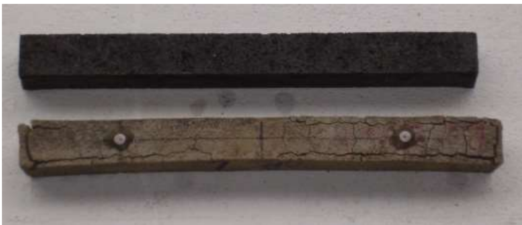
Fig. 7: Evident cracks and elongation of plain aerated concrete mortar bar (greyish specimen) in contrast to mortar bar containing palm oil fuel ash (black specimen)
