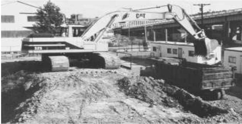
Fig. 1: A Caterpillar 325 Hydraulic Excavator (HEX)
