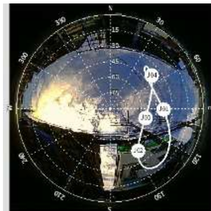
Fig. 5: Example of a sky image and the QZSS constellation. (Phuket, Epoch: September 1, 2025, 00:00:00 UTC, calculated using Rtklib[8])
