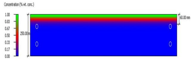
Fig. 6: Chloride Concentrations vs. Platform Depth (mixture 4 – 41.2 years)
