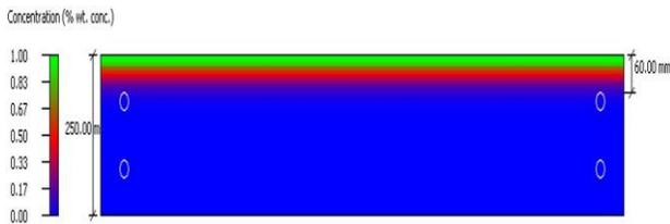
Fig. 5: Chloride Concentrations vs. Platform Depth (mixture 3 – 33.2 years)
