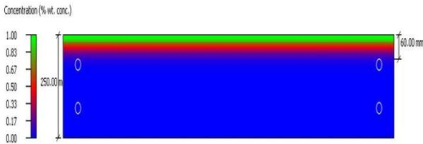
Fig. 7: Chloride Concentrations vs. Platform Depth (mixture 5 – 51.4 years)
