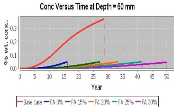
Fig. 10: Chloride Concentration vs. Time for the Six mixtures
