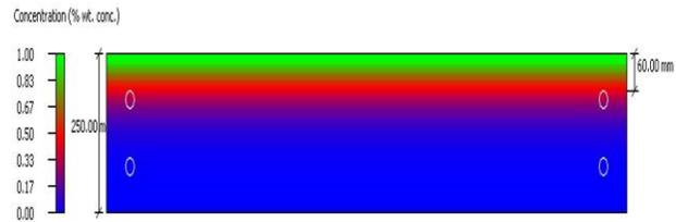
Fig. 8: Chloride Concentrations vs. Platform Depth for the Base Case (mixture 6 – 28.6 years)
