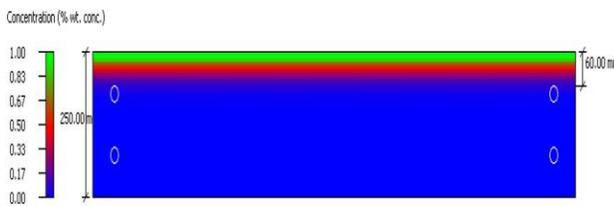
Fig. 3: Chloride Concentrations vs. Platform Depth (mixture 1 – 16 years)
