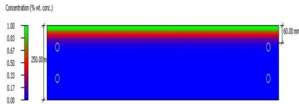
Fig. 4: Chloride Concentrations vs. Platform Depth (mixture 2 – 27.1 years)
