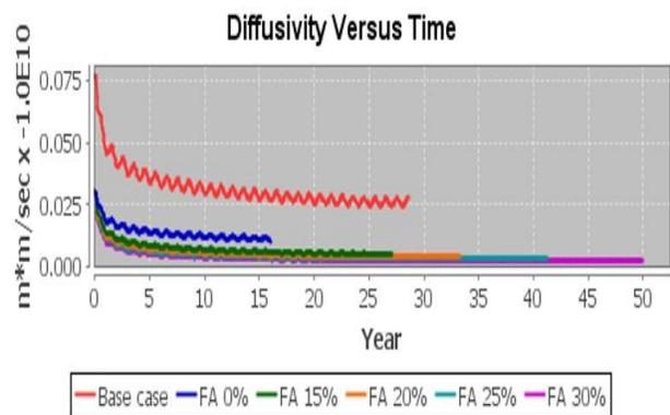
Fig. 12: Chloride Diffusivity vs. Time along the Corrosion Initiation Period
