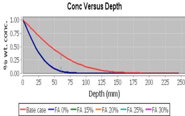
Fig. 9: Chloride Concentration vs. Depth for the all mixtures
