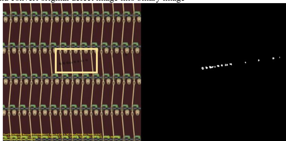
Fig. 2: Original Defect Image (Left) and Binary Image after Background Pattern Elimination (Right)
