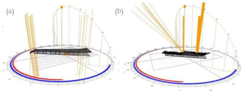
Fig. 5: Roof performance in reflecting solar radiation. (a) Original roof. (b) New inspired roof. (Ecotec Analysis 2011).
