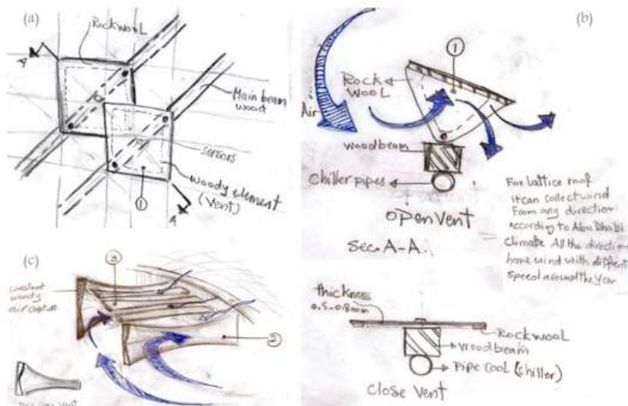
Fig. 3: Inspired roof's details. (a) Plan view of the dynamic woody elements- part no.1. (b) A cross section of the woody element in open and close conditions. (c) Pinecone vents as constant wind catcher – part no.2, and the sensitive louvers- part no. 3. (Source: Author).
