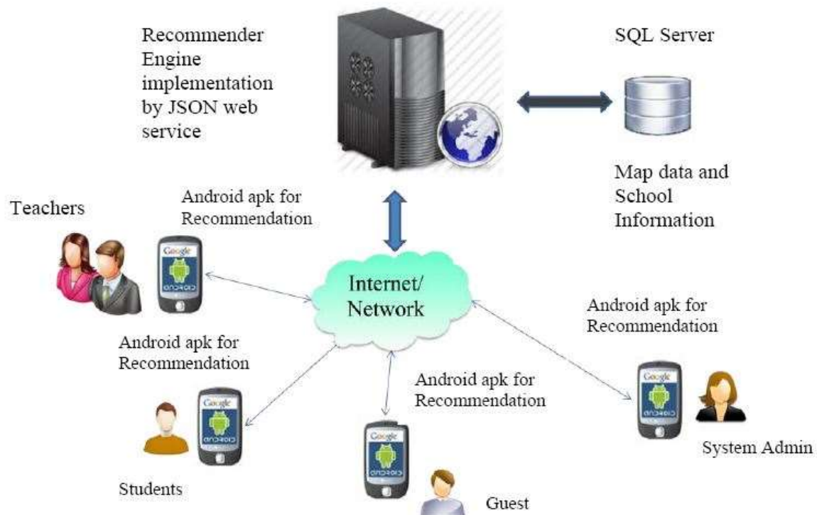
Fig. 1: System Architecture Design
